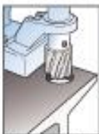
Cutting in I-beams
