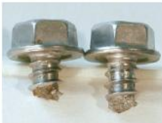
410 SS super passivated fastener with plain finish
