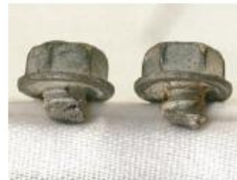
410 fastener with aluminum-filled topcoat
